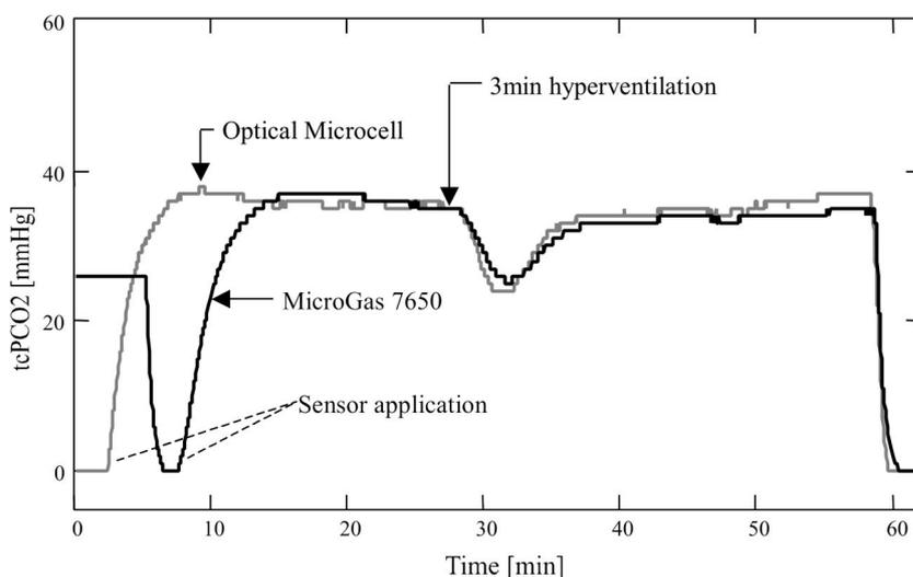
commercially available electrochemical transcutaneous sensor (MicroGas 7650, Radiometer-Basel, Switzerland) (Fig. 4).
